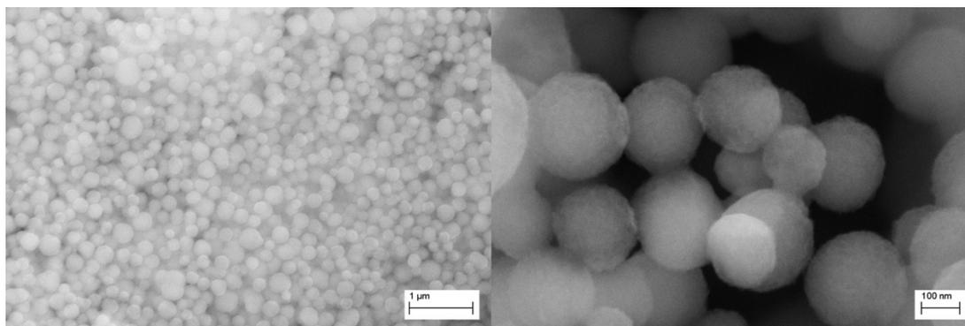
Figure 1. SEM micrographs of the bioglass nanoparticle sample with nominal composition 85% Si : 15% Ca at two different magnifications.
