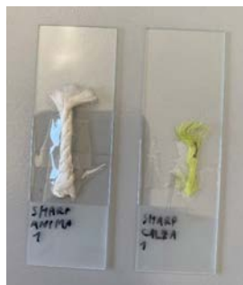
Figure 2 Core (white fibre) and sheath (yellow fibre) of a climbing rope broken with the UIAA 101 protocol.
