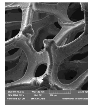
Commercial Ni Foam (pore size range 200 – 650 \mu\text{m} )
