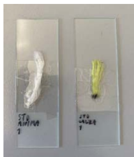
Figure 1 Core (white fibre) and sheath (yellow fibre) of a climbing rope broken with the EN 892 protocol.
