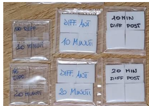
Figure 1. Sets of 4 CR39 dosimeters prepared for neutron irradiation at different irradiation times, in the standard configuration (left), in the configuration with front-positioned diffuser material (centre) and in the configuration with the back-positioned diffuser material (right).
