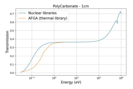
Neutron transmission, as a function of the incident energy of the particle, through a shielding layer of polycarbonate, as estimated using AFGA and compared to the nuclear libraries available at present.
